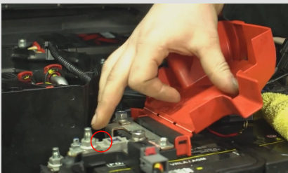
Figure O - Positive Unichip Terminal goes here (lower bolt).
