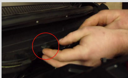
Figure B - Trim Fastener Removal
