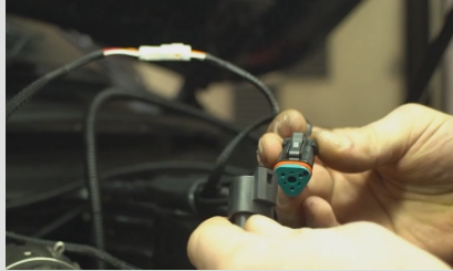
Figure N - Connecting Interior Wires to the Wiring Harness.
