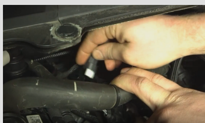
Figure G - Unclipping the Cam Shaft Sensor.
