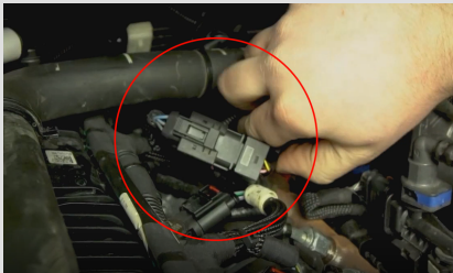
Figure I - Complete the connection with your existing sensor plug.
