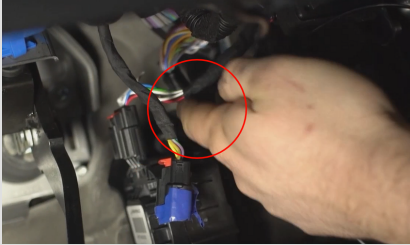
Figure M - Throttle Plug Position.
