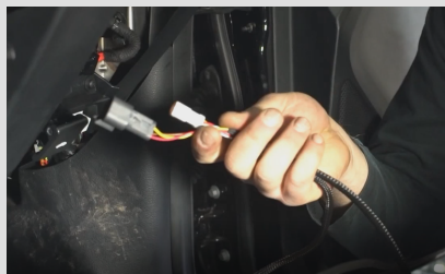
Figure L - Shown: Throttle & Map Switch wires.
