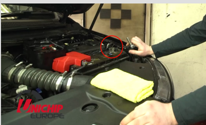
Figure A - Negative Battery Terminals
