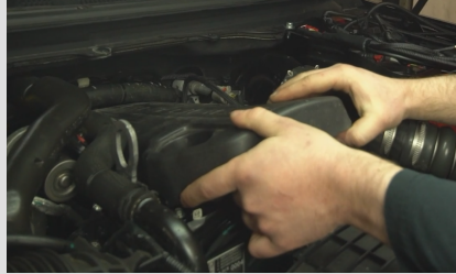
Figure D - Engine Cover Removal.
